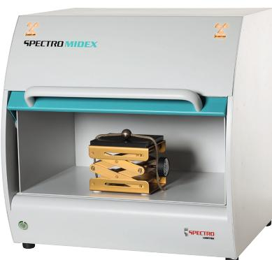
The SPECTRO MIDEX is known to be an all-round talent for the fast, non-destructive analysis of small spots in research and development, compliance screening and precious metals applications. It offers fast and extremely sensitive, non-destructive measurements. In addition, the SPECTRO MIDEX can also be used to analyze multi-layer structures for the layer thickness and the composition.
